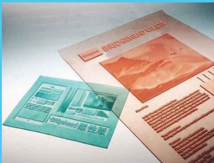
Old flexo plate with the rise image surface
